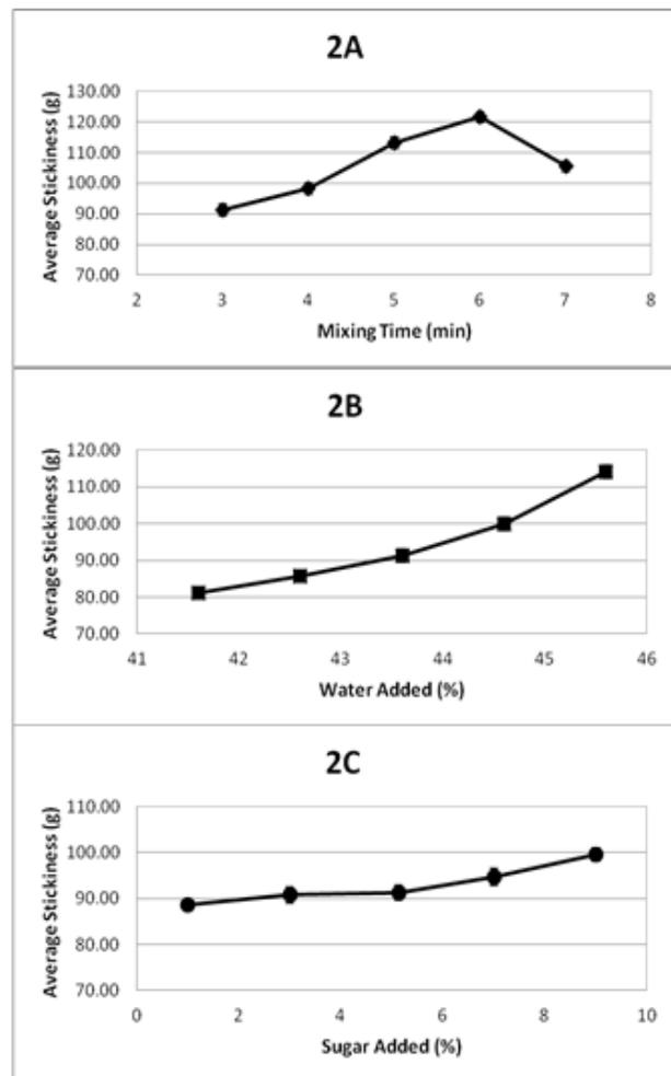
Figure 2. Effect of increment of (a) Mixing time (MT) (b) Water added (WA) (c) Sugar added (SA) on the average stickiness
